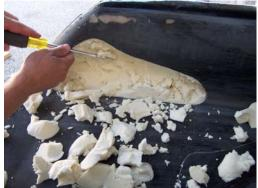
Using a screw driver, dig the foam until the foothold fit perfect.
