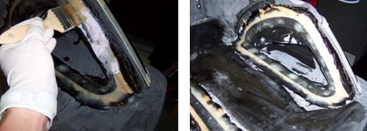
Using a paintbrush, apply the fiberglass with resin around the edges of the foothold and wait until dry.
