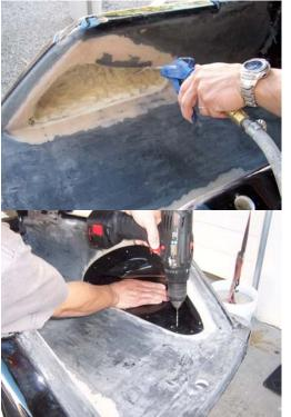
Put the foothold in the right place and drill the holes where you are going to put the screws.
