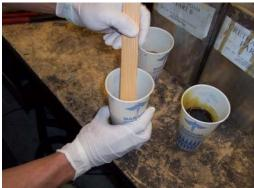
Using 2 part Foam, mix very well and insert into the top hole of the ski, to full the empty area.
