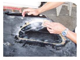
Using a sand paper #80, remove the excess.
