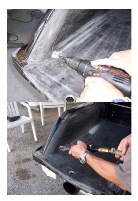
Using a drill, make a hole where you are going to star to cut.
