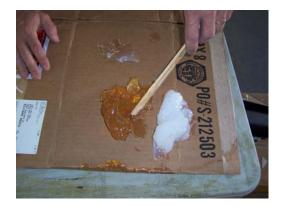
Using 2 part epoxy, mix both parts.
