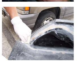
Using Epoxy Glue, close the hole where were the screws.
