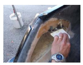
Apply epoxy glue in the back of the foothold and in the sanded area of the ski.
