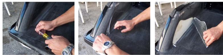
With a screw driver, remove fiberglass piece.
